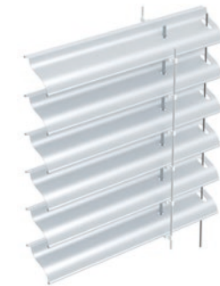
with wire tensioning, opened by 45°
